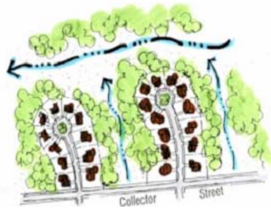
Figure 5.3-5 Natural drainage features can guide the design
